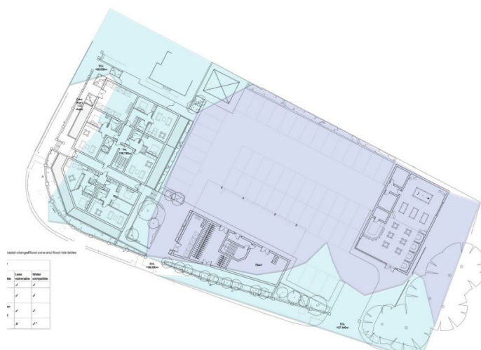
Figure 12: Overlay of development within flood zones
